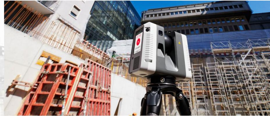
Laser scanner Leica BLK 360 e RTC 360
